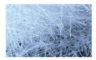
UHPC special synthetic fiber uses hydrophilic modification technology for its surface treatment. It has excellent dispersibility in UHPC, and has good bonding performance with cement matrix materials, which can effectively reduce and inhibit UHPC plastic shrinkage, drying shrinkage, Micro-cracks caused by temperature changes and other factors significantly improve crack resistance, toughening, impact resistance, fire and explosion resistance of UHPC.
