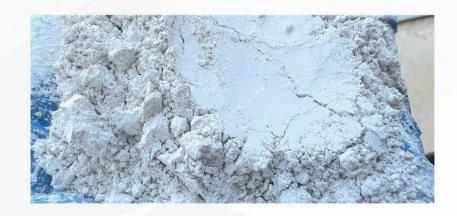
Ground Granulated Blast Furnace slag (GGBFS) is formed when GBFS is further processed and ground to a suitable fineness.
